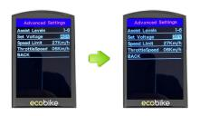
Set Voltage indicates the battery voltage bar (battery level) settings. Enter 5 voltage values one after the other. For example, VOL 1 is the first stage voltage value. The default value is 41.5 V.
