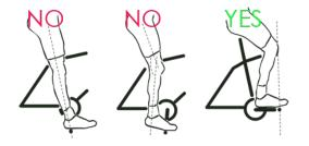
Please remember to set the saddle correctly (according to the figure below), it is important for the user because the incorrectly positioned saddle causes the cyclist to tire more quickly, pain in the legs and back.
