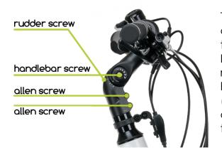
The handlebar, when placed in the most comfortable position for the user, must be tightened so that it does not loosen during riding. In an a-head type, the clearance should be removed by loosening the Allen screws on the handlebar bracket and tightening the rudder bolt (until the clearance is fully removed). After adjusting the bearings, tighten the Allen screws on the bracket - figure below.
